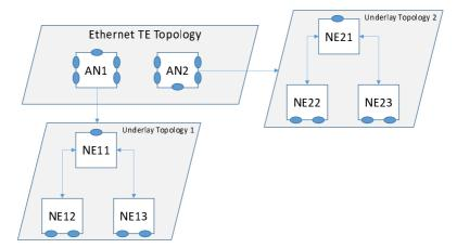
Figure 4.3.3.2.3.1: AL2 Ethernet Topology: Partial Connectivity, Use of Underlays
