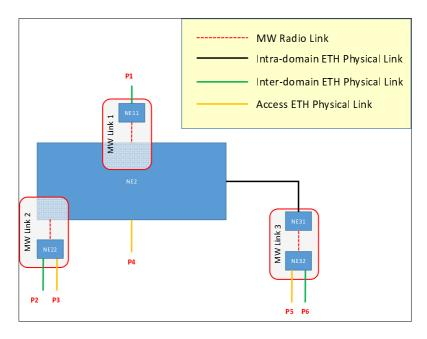
Figure C.1.1: Physical Representation of the Example Network
