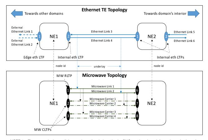
NOTE 1: The external ethernet links are shown for clarity only, the PNC needs to keep information only about the eeLTPs.
