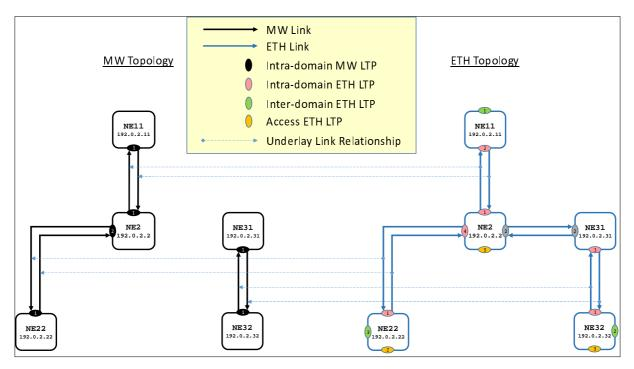
NOTE: The ltp-id values are local to the node, in this example they are (arbitrarily) numbered from 1 upwards, independently.
