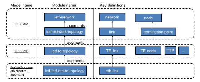
Figure 5.2.2.4.2: Ethernet Topology Model Hierarchy
